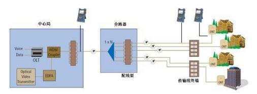
AV6416 Palm OTDR is mainly used to measure FTTx network, it provides a low cost solution for users.AV6416 offers three measuring modes: manual mode (including real time mode and average mode), auto mode and dead zone mode.
